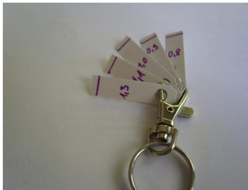
**Fig. 2.** Measuring ruler strips on a key chain for easy handling. Note that in Europe, a comma is commonly used instead of a decimal point. In this picture, the ruler is labeled with commas (eg, 1,3 IU rather than 1.3 IU).
